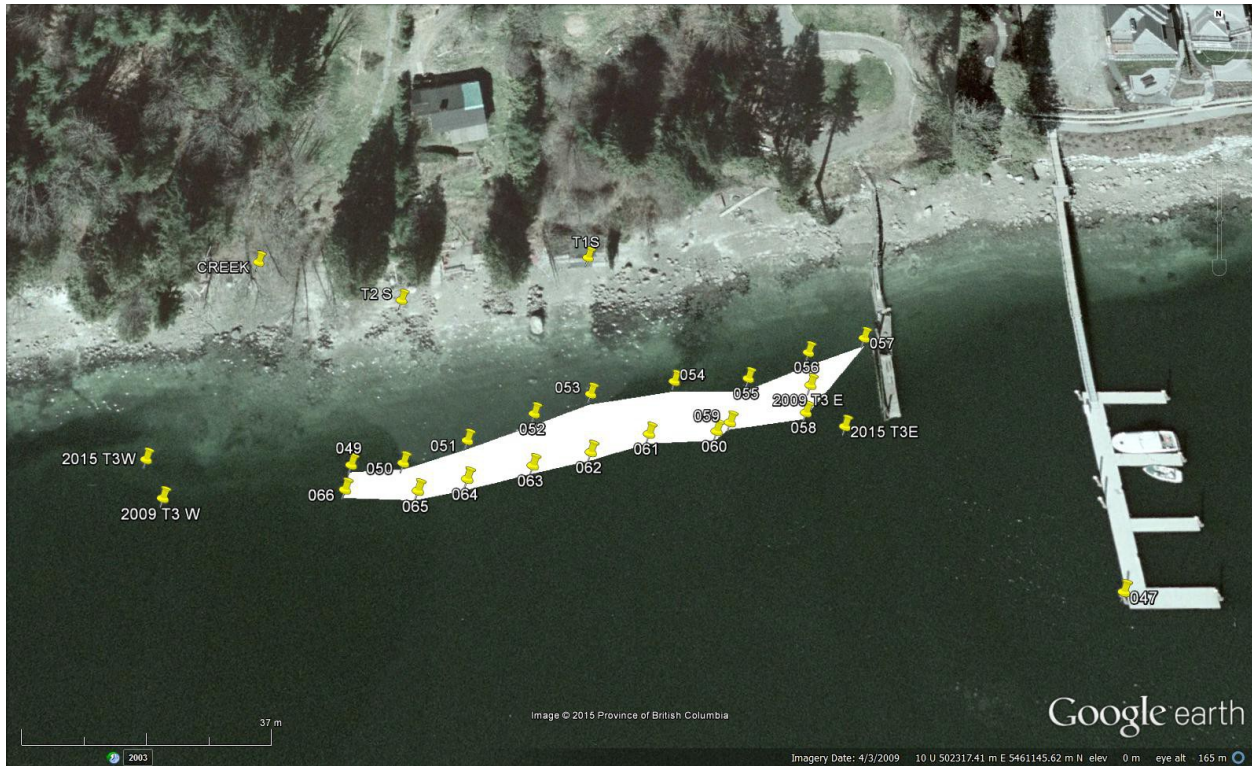
Illustration 2: GPS way points plotted onto an aerial image of the site. Lines connecting way points to create the polygon are interpolations.
